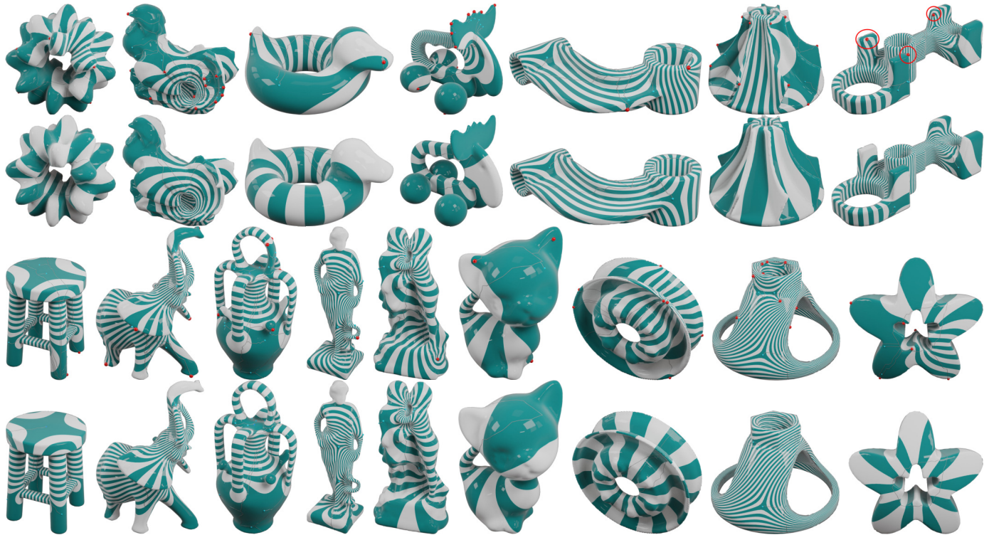
Fig. 31. Gortler-Thurston-Palmer’s Algorithm [7], [8] (1st, 3rd row) compared to ours (2nd, 4th row). Note the extra poles created by their algorithm, which are represented by red spheres and have been highlighted using red circles in the top-right figure.
