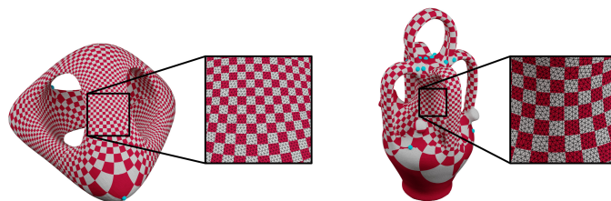
Fig. 15. With our multigrid solver, we can compute global conformal parameterizations on very large meshes, which cannot be achieved by [4].
